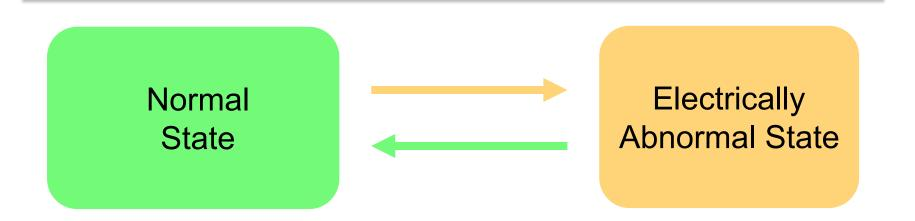
Operator must act to keep the system in the normal state or bring it back there if an incident takes it into the abnormal state
