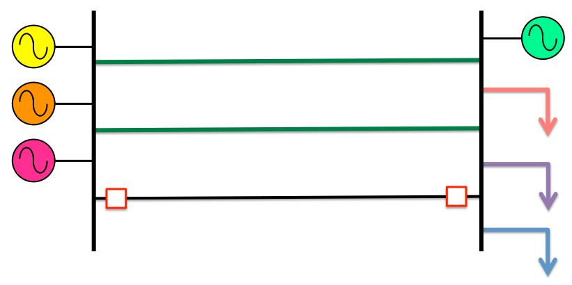
The system should remain stable following the loss of a single component
